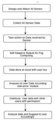
The RVNS-based Sensor Data Processing Framework (REDPF) offers an innovative solution to the challenges faced by healthcare IoT systems by integrating fog computing with advanced encryption techniques. The core components of the framework are designed to handle real-time data processing, ensure fault tolerance, and implement secure data encryption.
