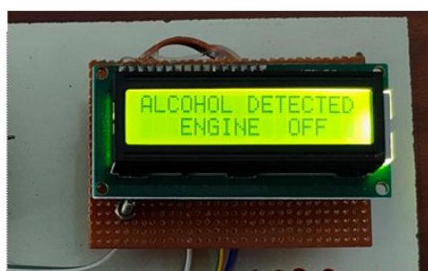
Fig: The LCD Module shows the alcohol detection
