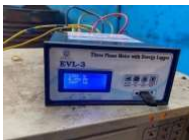
Figure 2: EVL-3 energy meter connected to the CNC milling machine
