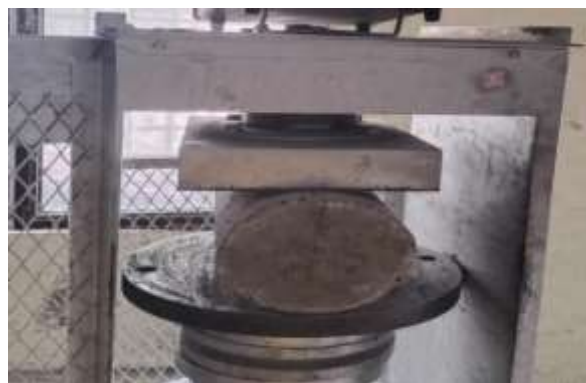
Fig. 8 Split Tensile Strength Test Setup
