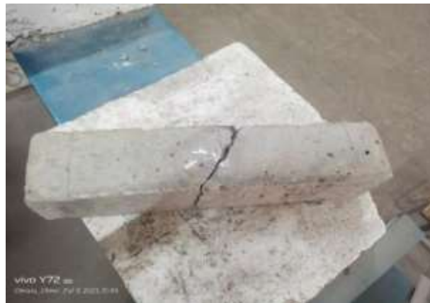
Fig. 10 Failure of Beam Specimen
