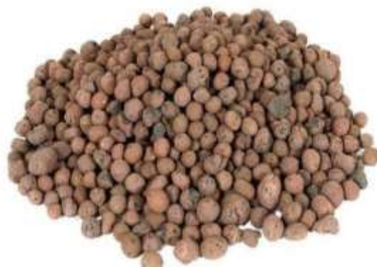
Fig. 1 LECA (Lightweight Expanded Clay Aggregate)
