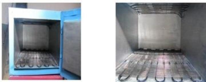
Figure 16: Assembly of insulated cabin and condenser mounting
