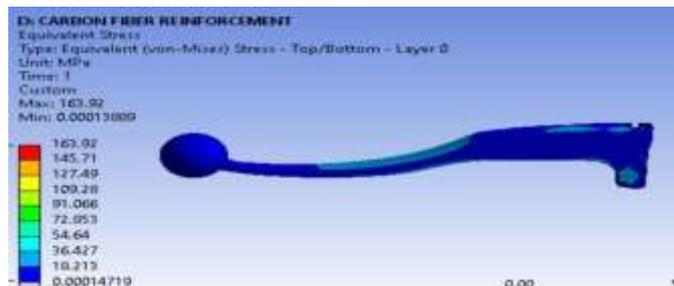
Fig. 27 Equivalent Stress of optimized hand brake lever with carbon fibre reinforcement
