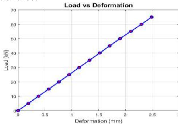
Fig. 12 Magnesium Alloy UTM Test Results
