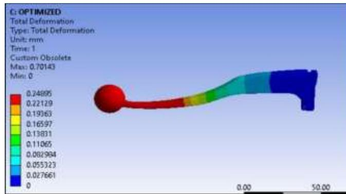
**Fig. 21 Total Deformation of optimized hand brake lever with Magnesium Alloy**
