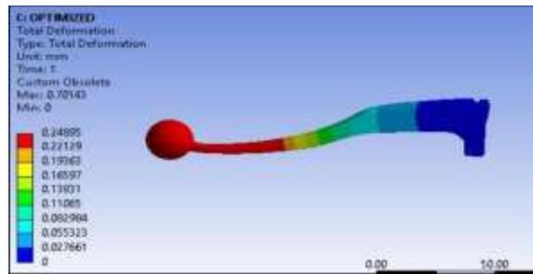
Fig. 15 Total Deformation of optimized hand brake lever
