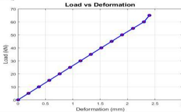
Figure 10 Aluminum Material UTM Test Results
