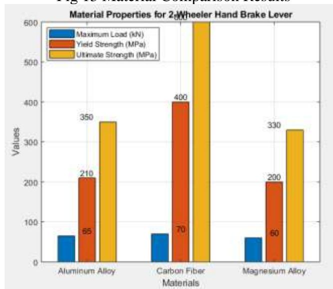
Fig. 14 Load Apply Different Material 2 Wheeler Hand Brake Lever
