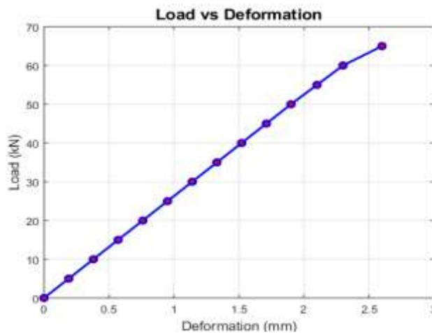
Fig 11 Carbon Fiber UTM Test Results
