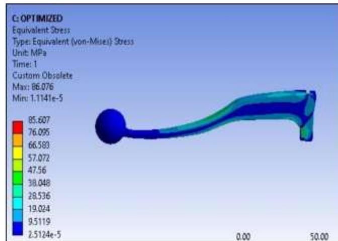
Fig. 16 Equivalent Stress of optimized hand brake lever
