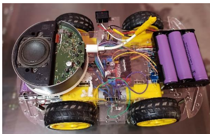
Fig 2.4.1: Prototype with final result (Design and Implementation of Smart Robot for Real Time Assistance in Disaster Management)
