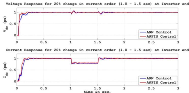
**Fig. 12 Voltage and Current Response of ANN and ANFIS Controller to 20% Step Change at inverter end**
