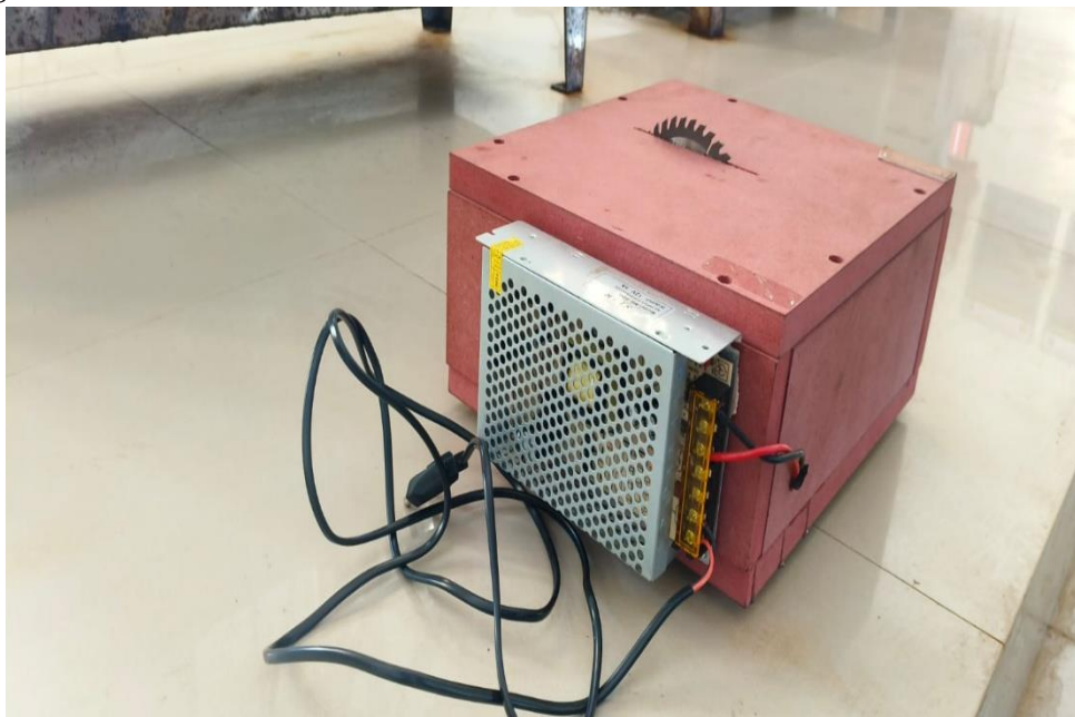
Figure 8: Final Assembly of Mini Table Saw
