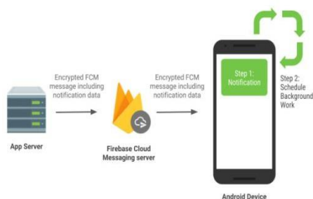
Fig.8: Cloud based system configuration
