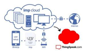
ThingSpeak is an open-source Internet of Things (IoT) application and API that allows for the storage and retrieval of data from sensors and hardware devices. It communicates using the HTTP protocol over either a LAN or the internet. MATLAB analytics is integrated to help analyze and visualize the data collected from hardware or sensor devices. Each type of sensor data can be assigned its own
