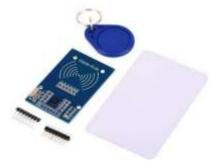
An RFID (Radio Frequency Identification) reader is a device that collects data from an RFID tag, facilitating the tracking of individual items. Unlike barcodes, RFID technology doesn't require a direct line of sight or scanning of the tag, which enhances the flexibility and efficiency of tracking.
