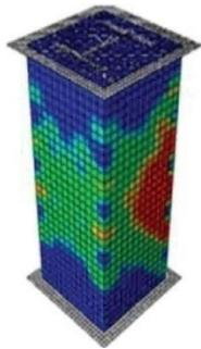
(Figure 7: Effects of concrete strength on damage characteristics of the encased composite column: (a)  $f_{ck} \diamond 25$ ; (b)  $f_{ck} \diamond 30$ ; (c)  $f_{ck} \diamond 35$ .)
