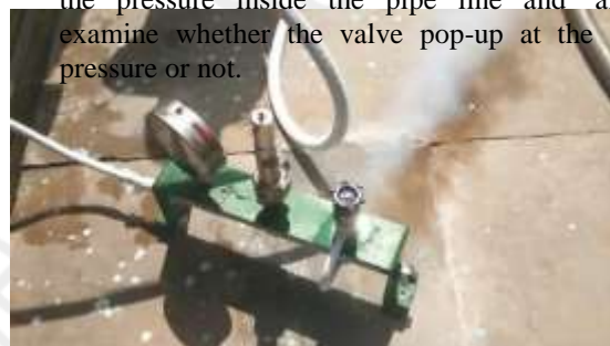
Fig. 4.4 Pressure Gauge – Globe valve setup
