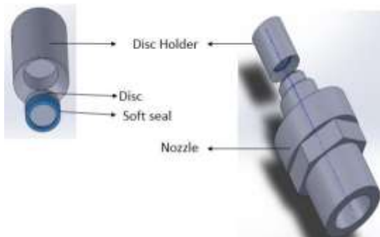
Fig. 5.1 Metal disc with disc holder and nozzle assembly
