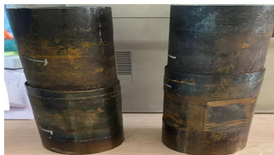
Figure 1: Friction welded joints of parent metals
