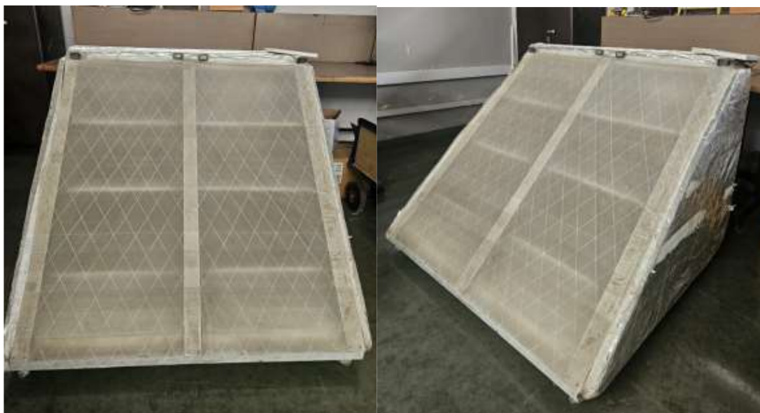
Figure 2 Direct type Domestic multi shelf dryer front and isometric view
