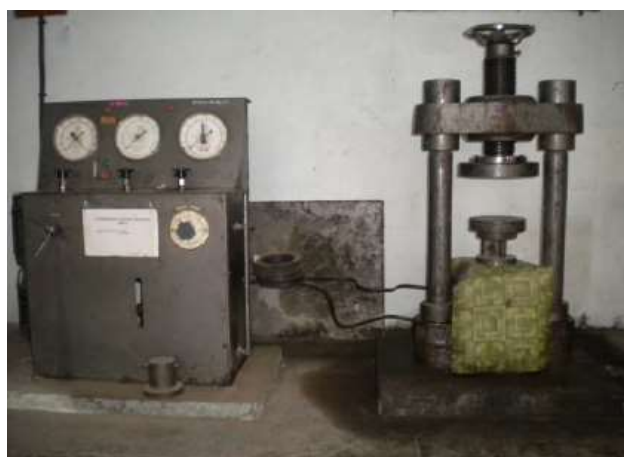
FIGURE 3: COMPRESSION TESTING MACHINE
