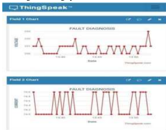
Fig:4.2.3 Real-time Monitoring of Voltage and Current Readings in ThingSpeak Website
