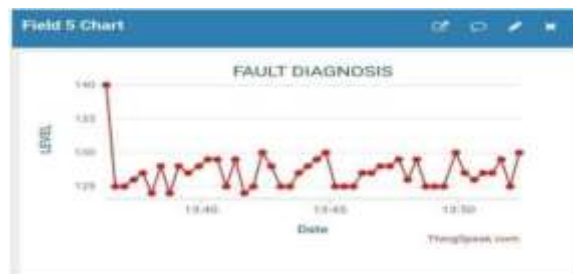
Fig:4.1.2 The Real-time Monitoring of Oil Level Readings in ThingSpeak Website
