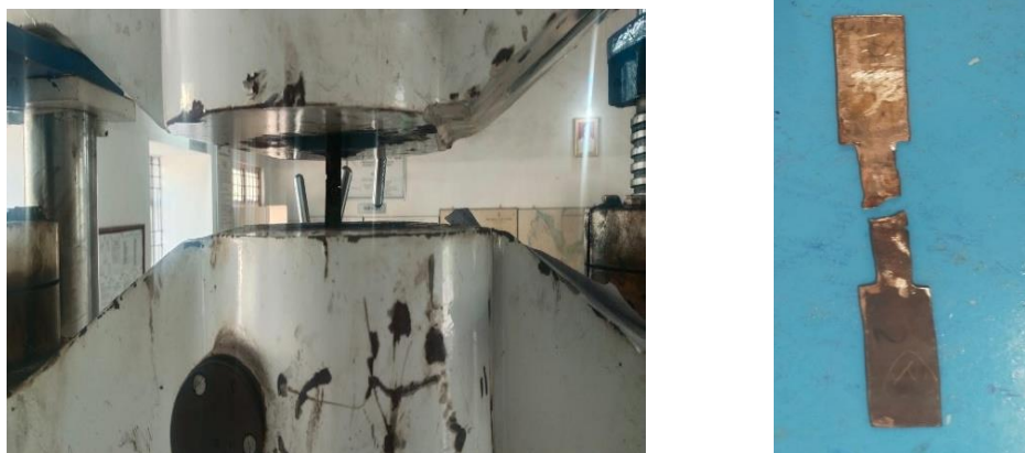
Fig. 4.3(b) Final Specimen after tested on UTM Machine for Tension
