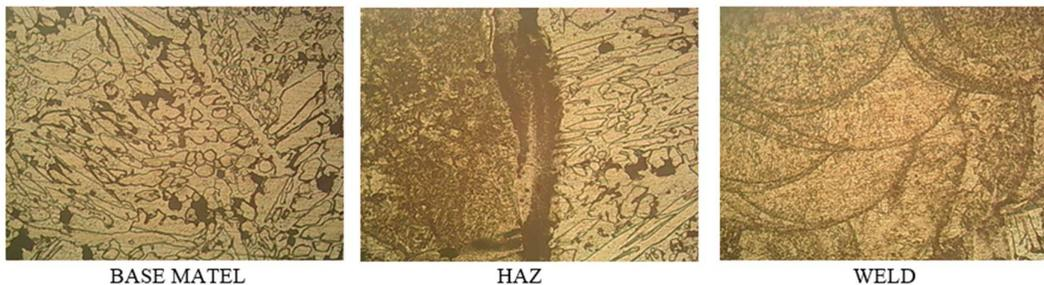
Figure 3: Cold rolled microstructure
