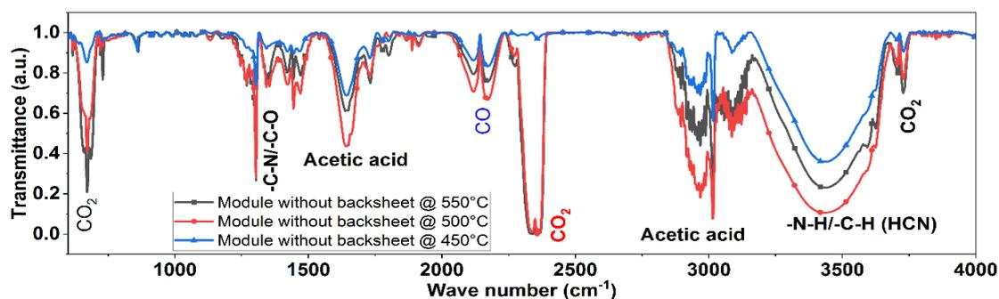
Figure 9. FTIR spectra of fume collected during pyrolysis of PV module without backsheet at 450°C, 500°C and 550°C [8]
