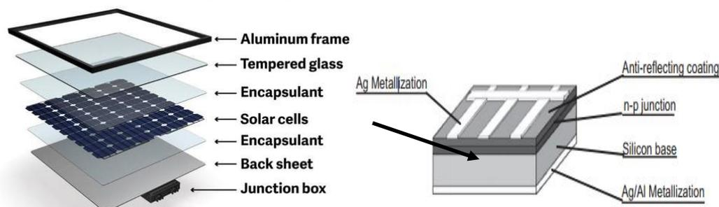
Figure 1. Solar module basic structure, and types of material used in solar cell [1].
