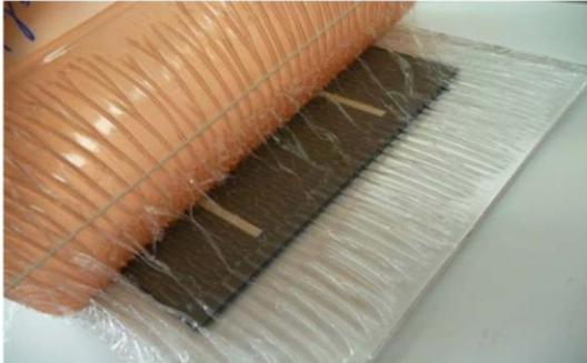
Figure 6: Removal of the back sheet from a Thermoplastic encapsulant based module [5].
