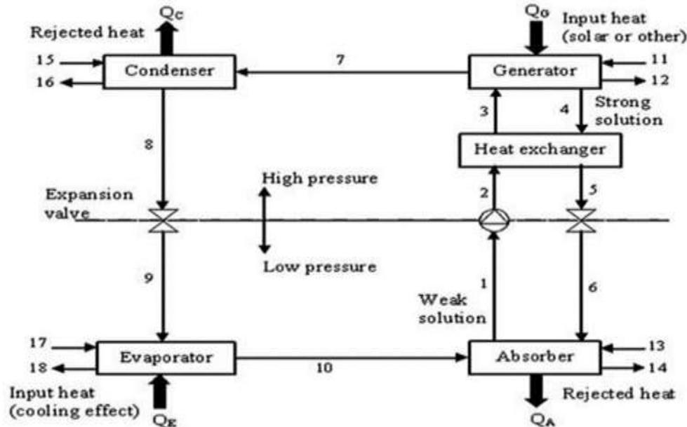
Figure 1 Schematic Diagram of Simple Vapour Absorption Refrigeration System
