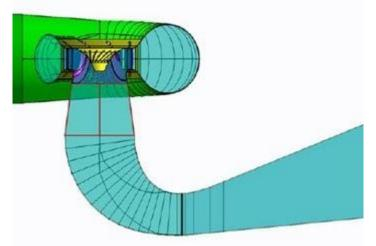
**6. Tailrace** Tailrace is the flow of water from turbines to the stream. It is good if the power house is located nearer to the stream. But, if it is located far away from the stream then it is necessary to build a channel for carrying water into the stream.
