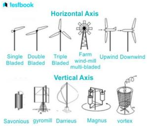
**Horizontal Axis Wind Turbines (HAWT):** These turbines resemble windmills, with the tip of the shaft pointing in the direction of the wind. Smaller turbines are steered by wind vanes mounted on the building since they must face the wind. Wind sensors and servos are used with larger turbines to turn them.
