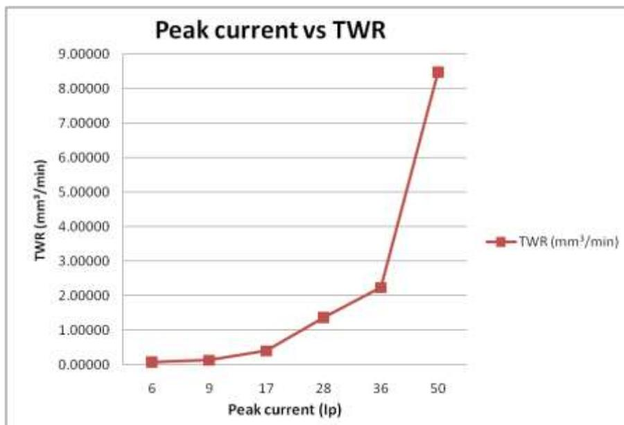
**Figure 6** Effect of variation in Peak Current on TWR at pulse on-time = 100  $\mu$ s, pulse off time = 96  $\mu$ s, and gap voltage = 50 V
