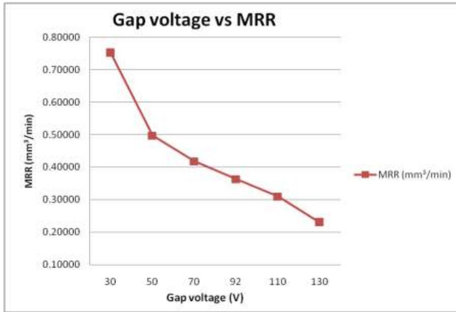
**Figure 5** Effect of variation in Gap voltage on MRR at pulse-on-time = 100  $\mu$ s, pulse off-time = 96  $\mu$ s, and peak current = 17 A
