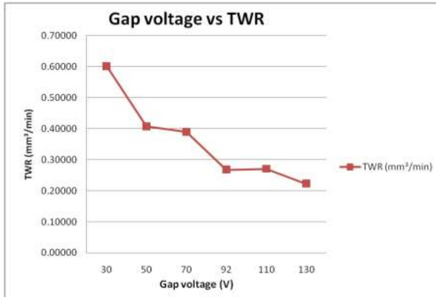
**Figure 9 Effect of variation in Gap voltage on TWR at pulse-on-time = 100  $\mu$ s, pulse off-time = 96  $\mu$ s, and peak current = 17 A**
