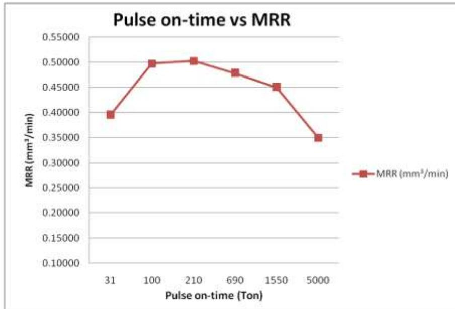
**Figure 3 Effect of variation in Pulse-on-time on MRR at pulse off-time = 96  $\mu$ s, gap voltage = 50, and peak current = 17 A**
