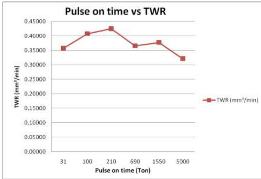
**Figure 7 Effect of variation in Pulse-on-time on TWR at pulse off-time = 96  $\mu$ s, gap voltage = 50, and peak current = 17 A**
