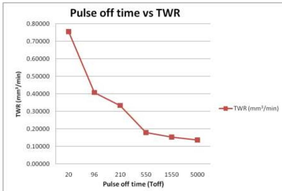
**Figure 8 Effect of variation in Pulse-off-time on TWR at pulse-on-time = 100  $\mu$ s, gap voltage = 50, and peak current = 17 A**
