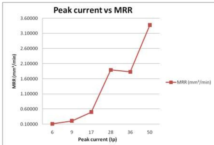
**Figure 2 Effect of variation in Peak Current on MRR at pulse on-time = 100  $\mu$ s, pulse off time = 96  $\mu$ s, and gap voltage = 50 V**
