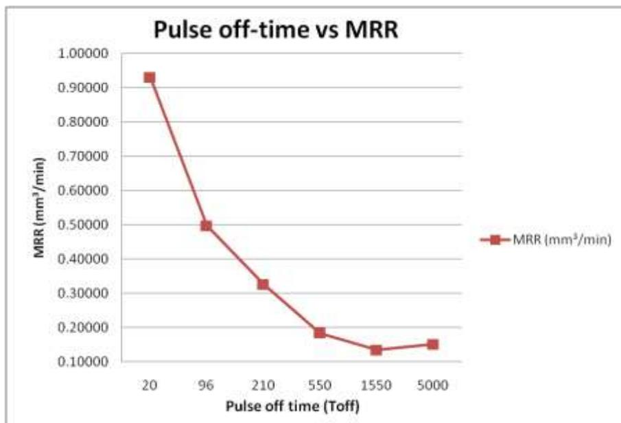
**Figure 4 Effect of variation in Pulse-off-time on MRR at pulse-on-time = 100  $\mu$ s, gap voltage = 50, and peak current = 17 A**
