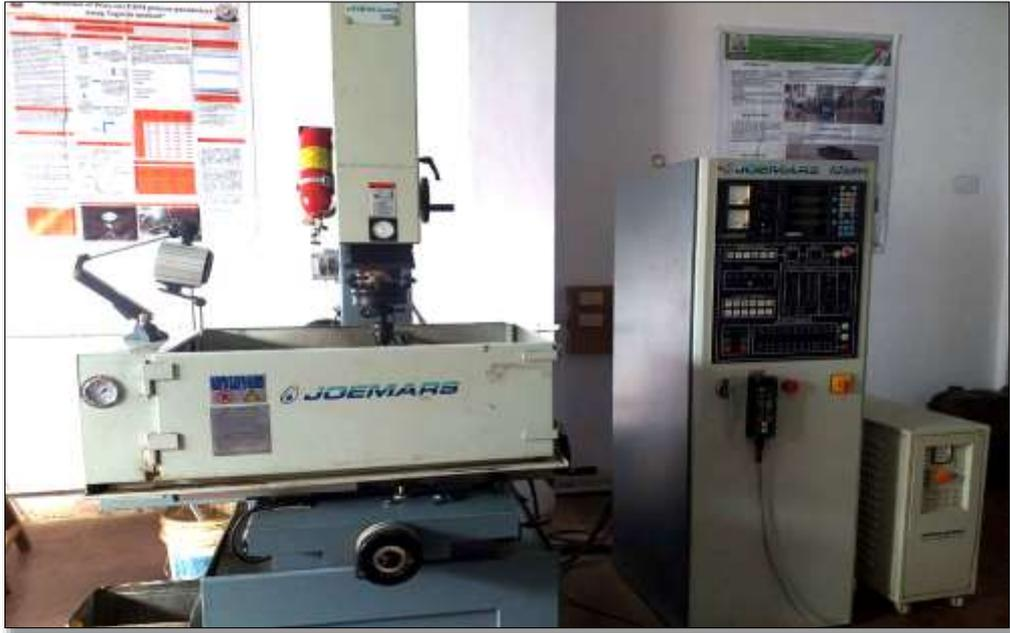
Figure 1 A pictorial view of the EDM machine along with Fuzzy-controller
