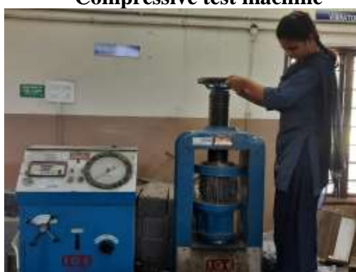
Placing of cube in ucs machine
